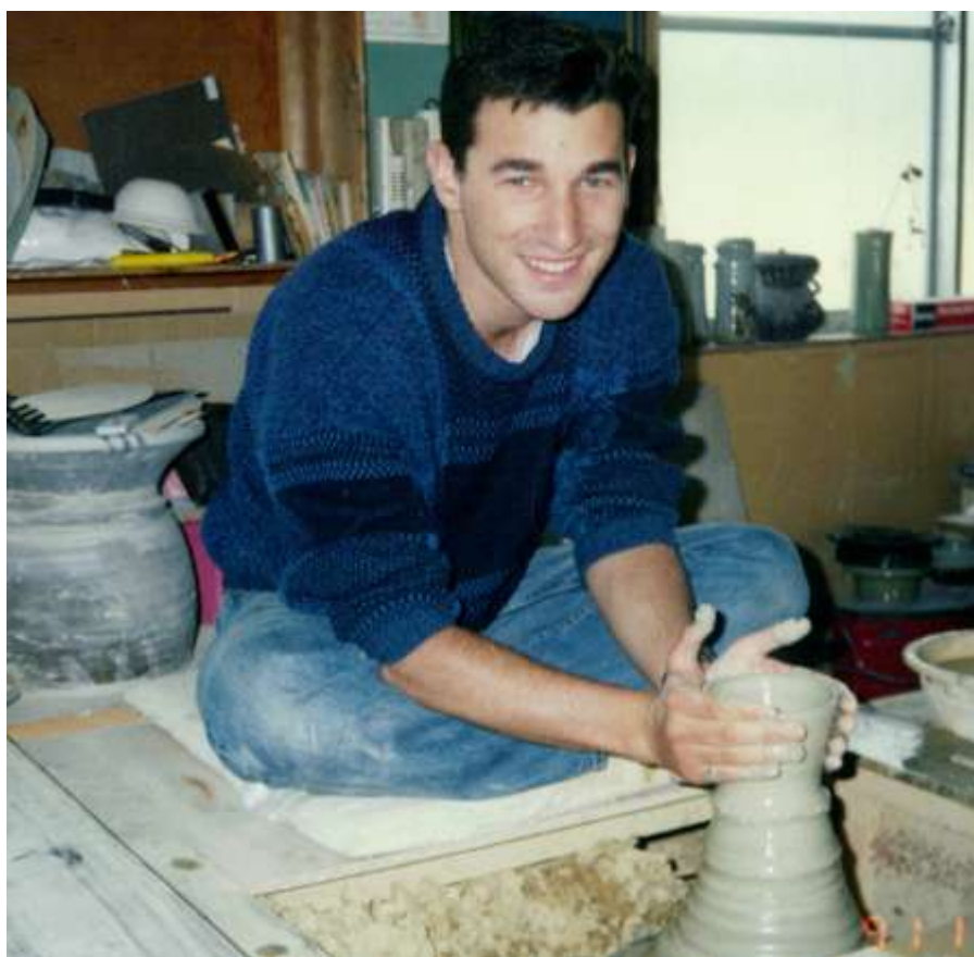
Beginning the pottery-making process. Getting the lump of clay to rotate perfectly around the center axis is far, far harder than it looks in the movies.
